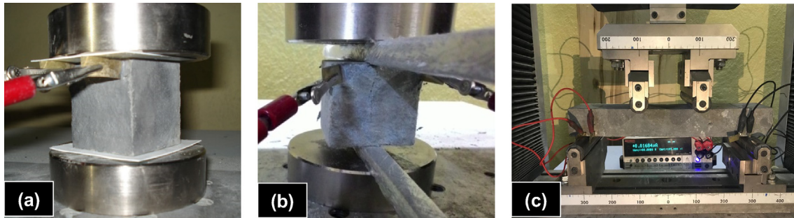
Fig. 2. Proposed configurations for ER measurements under (a) uniaxial compression (b) splitting tensile and (c) four-point bending loading.
