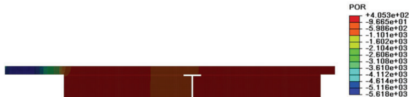
Figure 9. Sound pressure FEA result of the silencer with an extension tube.
