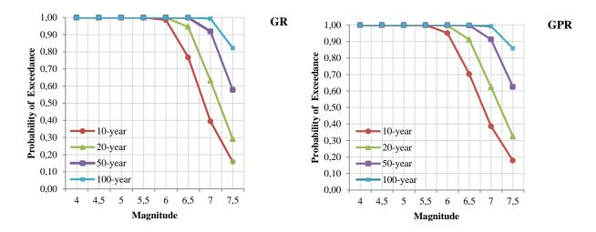
Figure 4. The probability of exceedence graphs for GR and GPR models
