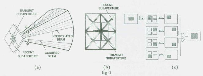
(a) Volumetric imaging. (b) Mills cross array configuation. (c) Aperture space representation of transmerceive subapertures (K=2) and their sum.
