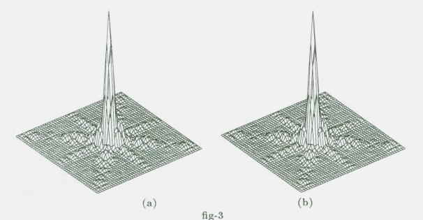
(a) Proposed technique psf and (b) Control psf. (Lateral axis:  $sin\theta$ , Elevation axis:  $sin\phi$ , vertical amplitude.) For figure 3:  $(K = 2, N_t^x = N_t^y = 16, N_r^x = N_r^y = 16, B^{\theta} = B^{\phi} = 24, B^{\theta}_o = B^{\phi}_o = 48.)$
