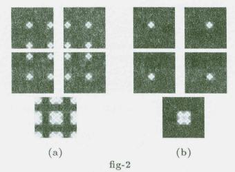
(a) Equivalent subapertures are viewed periodic and their sum before linear filtering. (b) Equival subapertures and their sum after linear filtering.
