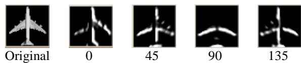
Figure 6. An aircraft image and 2D Gabor filter outputs in four orientations (0, 45, 90, and 135 degrees).
