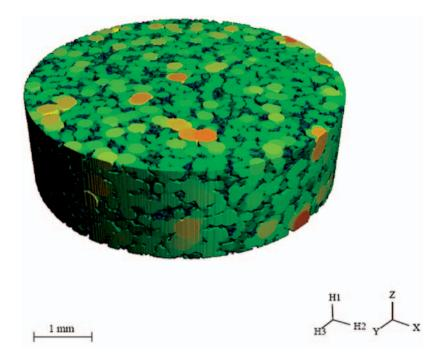
Figure 1. A representative µ-CT image of the PLLA/PCL blend scaffolds
