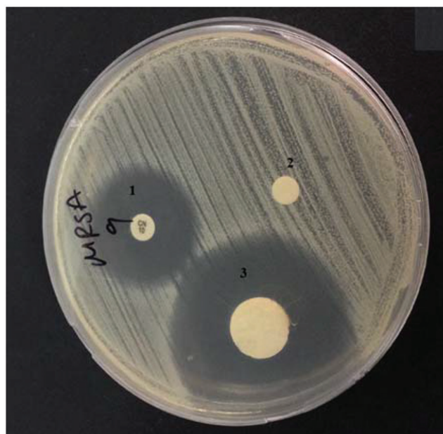
Figure 1. Discs in agar medium (1) antibiotic disc, (2) empty disc, (3) antibacterial polymer.
