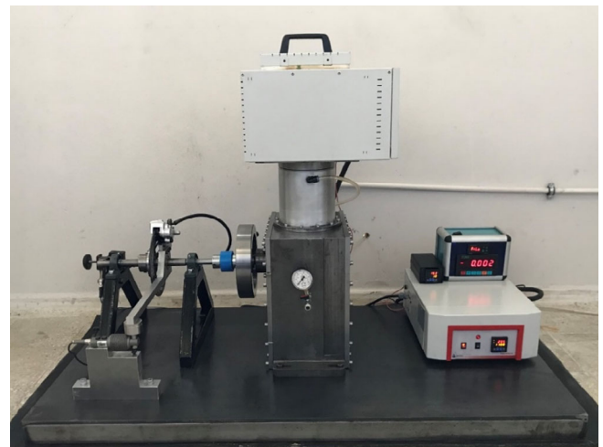
FIGURE 10 View of the experimental setup of Stirling engine and measuring devices [Colour figure can be viewed at wileyonlinelibrary.com ]
