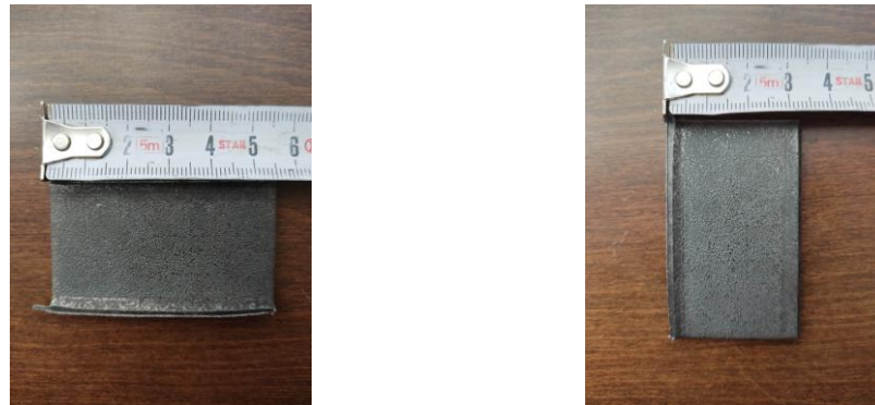
Figure 1. Scrap sample for spectral analysis (Scrap 5, 5.5 × 3 cm).
