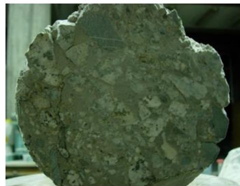
Fig. 1. A sample of PAC prepared by the new SCG method
