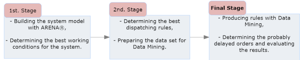
Figure A. Stages of the model for estimation of probably delayed orders in job-shop production with data mining
