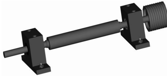
Figure 2. Shaft-Ball bearing experimental arrangement (Karacay and Akturk[27])
