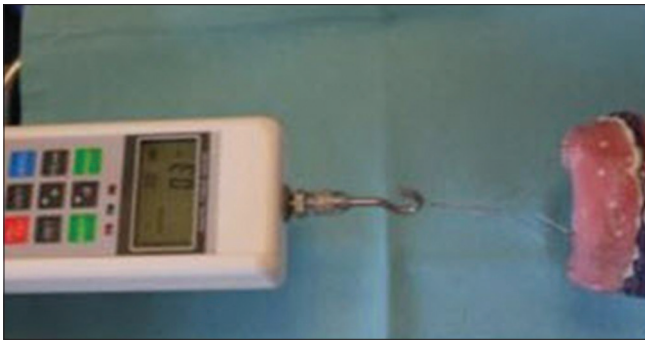
Figure 7: Connection of the digital dynamometer to the impression tray with orthodontic ligature wire
