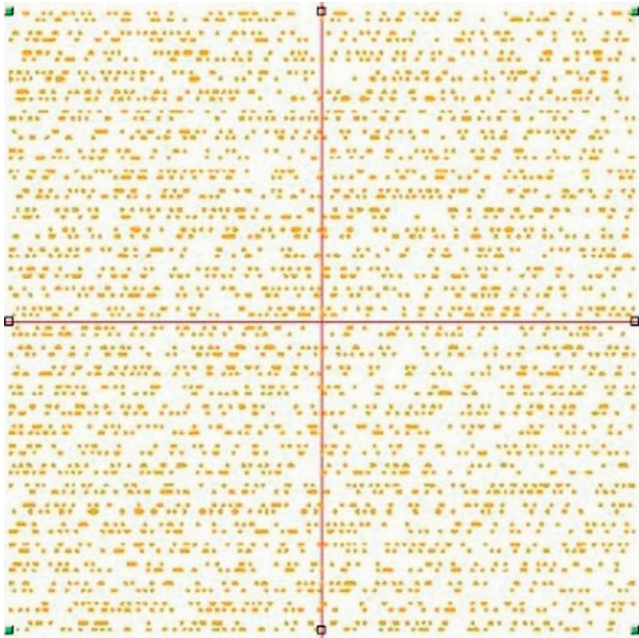
Figure 1. The standard roughening pattern used by femtosecond laser.
